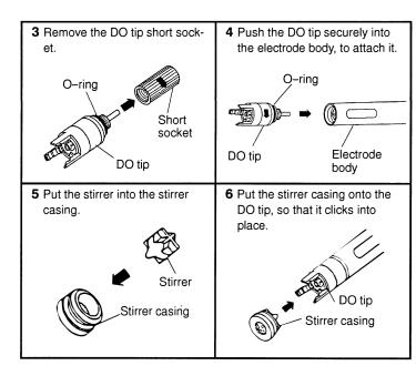
Note ▶▶▶ Do not dispose of the short socket that was removed. It is necessary when storing the electrode.
