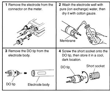
Note ▶▶▶ Avoid storing the electrode in a hot place or places with high humidity. Store the electrode indoors, out of direct sunlight.
