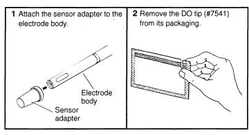
Note ▶▶▶ An O-ring is attached inside the sensor adapter, so push the sensor adapter in with a little force, while turning it.
